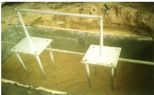
Figure 2.3: Model plane frame at base setup load
