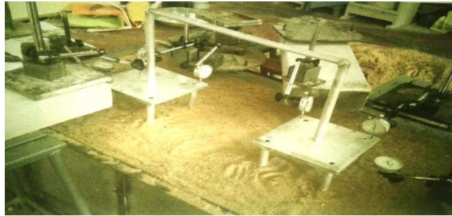
Figure 2.5: Model plane frame arrangement of dial gauge
